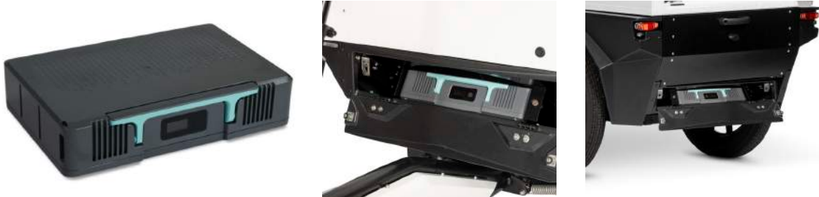
Figure 12: Location of the two LiFePO 4 batteries. One on the front side and one on the rear side of the bike.
